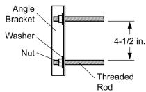
condition, the main limit imposed by the scoreboard is that the posts have to fit inside the mounting clamps (assuming you wish to use the hardware provided by Electro-Mech). The standard clamps form a "pocket" that is 4-1/2 inches square. So, if you try to use a 10-inch diameter pipe, our clamps will not work.
